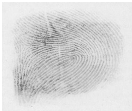
FIG. 3—Cyanoacrylate-developed latent fingerprint on polyethylene dinner plate stained with Janus green B.
