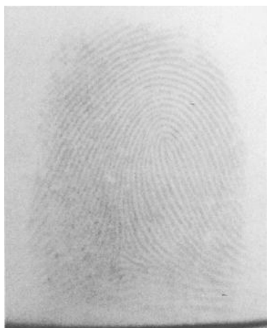
FIG. 6—Cyanoacrylate-developed latent fingerprint on polyethylene dinner plate stained with dark green Rit fabric dye.
