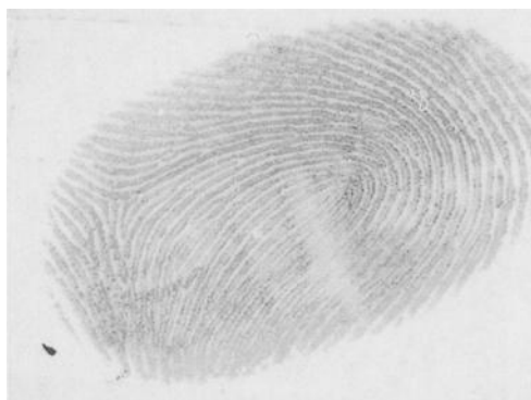
FIG. 1—Cyanoacrylate-developed latent fingerprint on polyethylene dinner plate stained with gentian violet.
