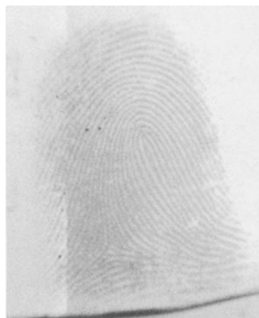
FIG. 7—Cyanoacrylate-developed latent fingerprint on polyethylene dinner plate stained with scarlet Rit fabric dye.
