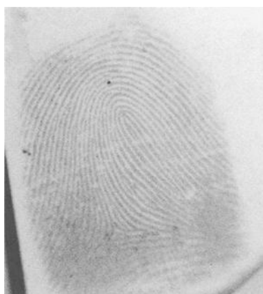
FIG. 5—Cyanoacrylate-developed latent fingerprint on polyethylene dinner plate stained with dark brown Rit fabric dye.
