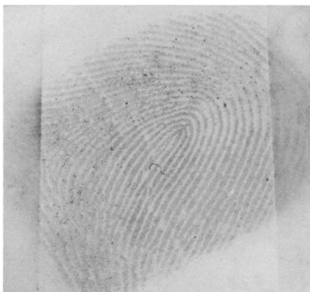
FIG. 4—Cyanoacrylate-developed latent fingerprint on polyethylene dinner plate stained with black Rit® fabric dye.
