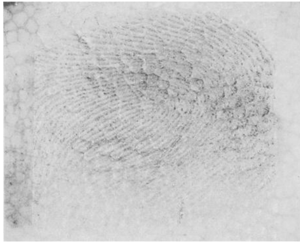
FIG. 8—Cyanoacrylate-developed latent fingerprint on Styrofoam cup stained with navy Rit fabric dye.
