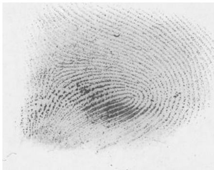
FIG. 9—Cyanoacrylate-developed latent fingerprint on porcelain bowl stained with black Rit fabric dye.
