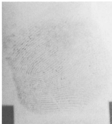
FIG. 10—Cyanoacrylate-developed latent fingerprint on aluminum beverage can stained with black Rit fabric dye.
